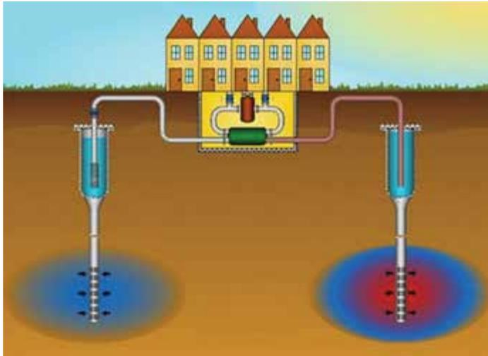
The cold and heat are added to the water by means of a heat exchanger. That could be, for example, the roof of a building under which water pipes run, absorbing the heat and cold. If the cold water is not at the right temperature in the summer, and if the warm water is not at the right temperature in the winter this can be rectified with the aid of a heat pump.
