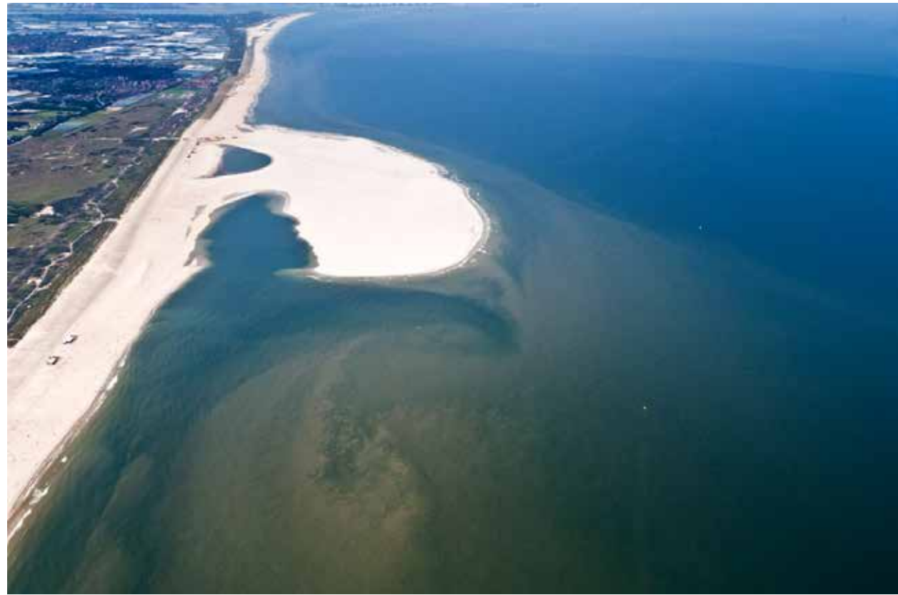
Figure 1. Aerial image of the Sand Motor just after construction. The sediment clouds at the water surface clearly show the presence of a tidal eddy as a result of flow separation.
