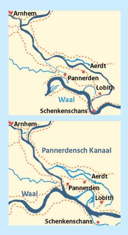
How the Pannerdensch Kanaal restored discharge patterns via the Lower Rhine and the IJssel.
