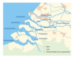
Where flow rates at Lobith fall below 1100  $m^3/s$ , the Haringvliet lock complex is shut completely, with the exception of the saline outfall and fish pass. Where flow rates in the Rhine are between 1100 and 1700 m<sup>3</sup>/s, a small flushing opening  $(25 \text{ m}^3/\text{s})$  is used where the level of the external waters is lower than that of the internal waters. In this way, the flushing rate in the western part of the Haringvliet is an average of approx. 50 m<sup>3</sup>/s per tide.
