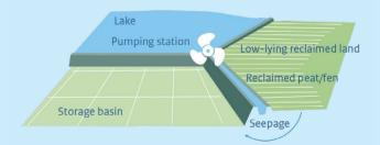
Schematic diagram of a polder and land reclaimed from a body of water.
