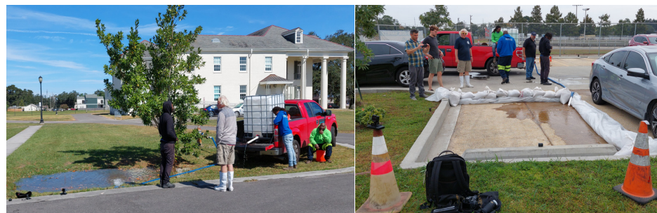
Figure 5. (Left) FSIT at raingarden Milne (test number G14, Table 1). (Right) FSIT at permeable pavement after building a confined space with plastic and sandbags.
