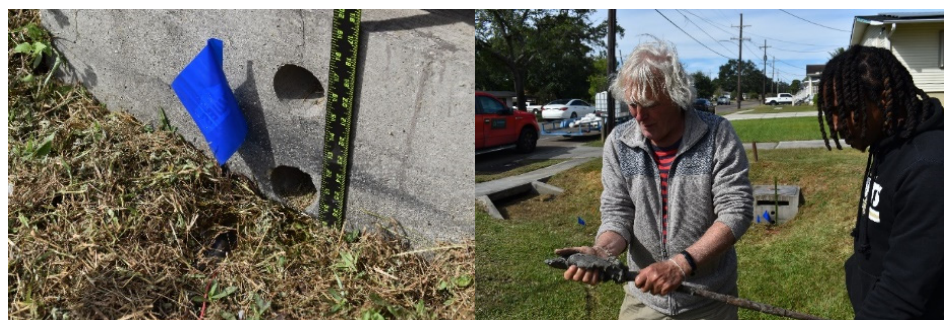
Figure 6. Measurement with loggers and rulers (left) and additional information by drilling the soil (right).
