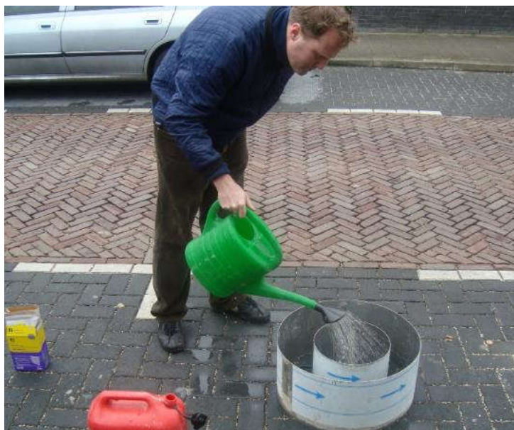
Figure 4. Double-ring infiltrometer tests.
